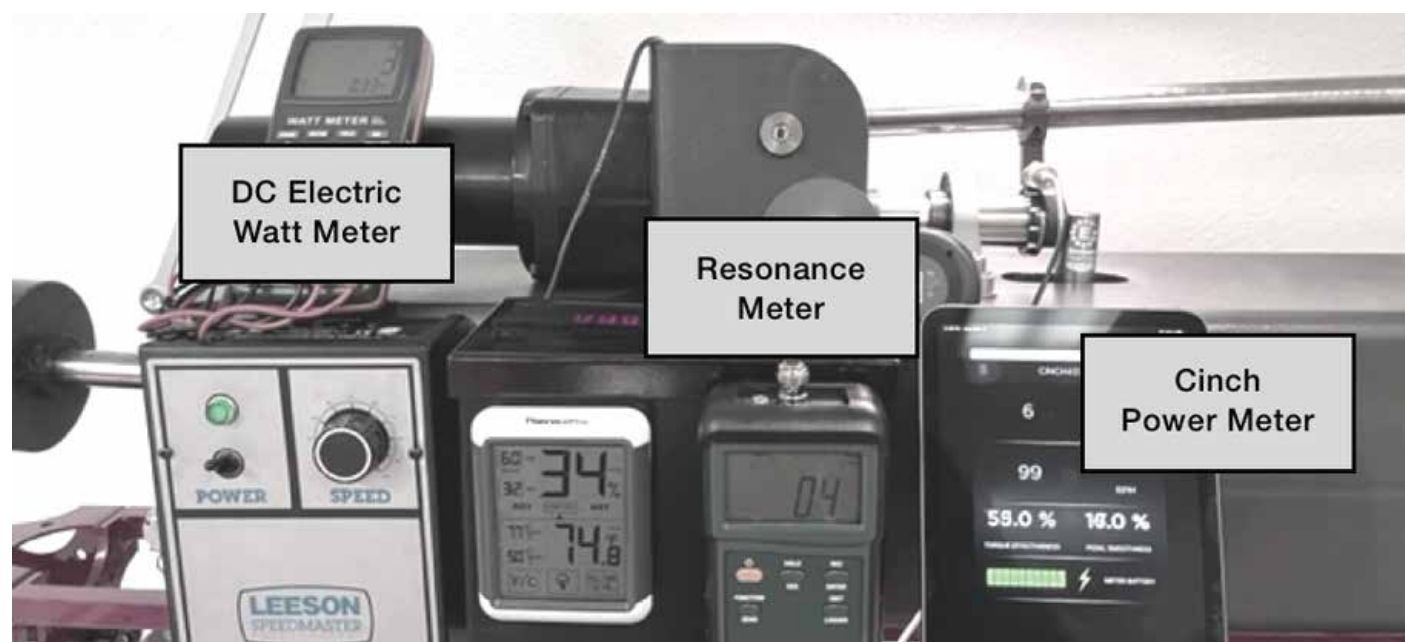
■ Testing setup for the Enduro Bearings XD15 bottom bracket bearing
